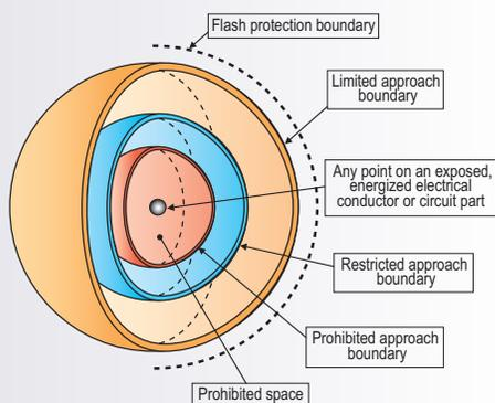
**Flash protection boundary** – distance within which a person could receive a second degree burn if an electrical arc flash were to occur. Persons inside this boundary must use appropriate, flash-flame protection equipment.
